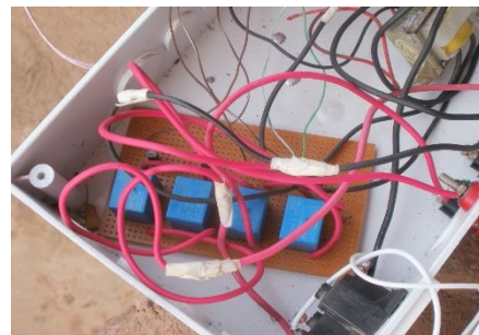
Figure 8: Power Supply and Relay Connection
