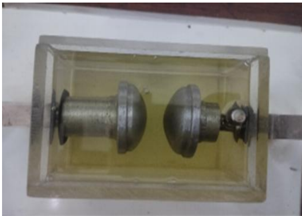
Figure 1 Mushroom – Mushroom Electrode Configuration
