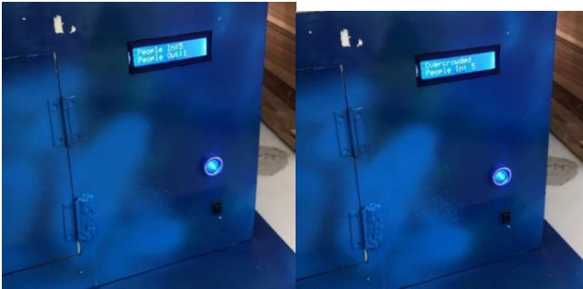
Figure 4: Enclosed prototype displaying occupancy on LCD.
