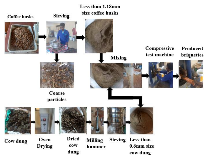
Figure 1: Process flow for producing coffee-husk briquettes with cow-dung binder
