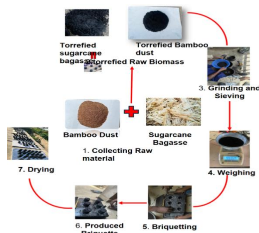
Figure 2: Biomass Preparation and and Briquetting Process
