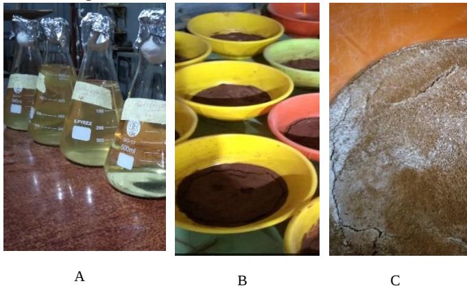
Figure 1. (a) Bacillus thuringiensis solution (b and c) prepared samples with bacterial and cementation solutions for consistency limits.
