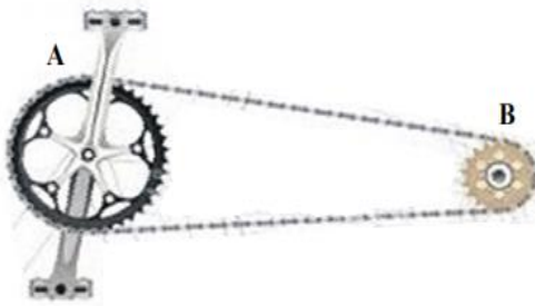
Figure 3b: Gear train of the pedal-operated generator. A driver gear (44 teeth) drives a smaller gear (18 teeth) via a chain to increase rotational speed. Adapted from Ikechukwu and Anthony [19].
