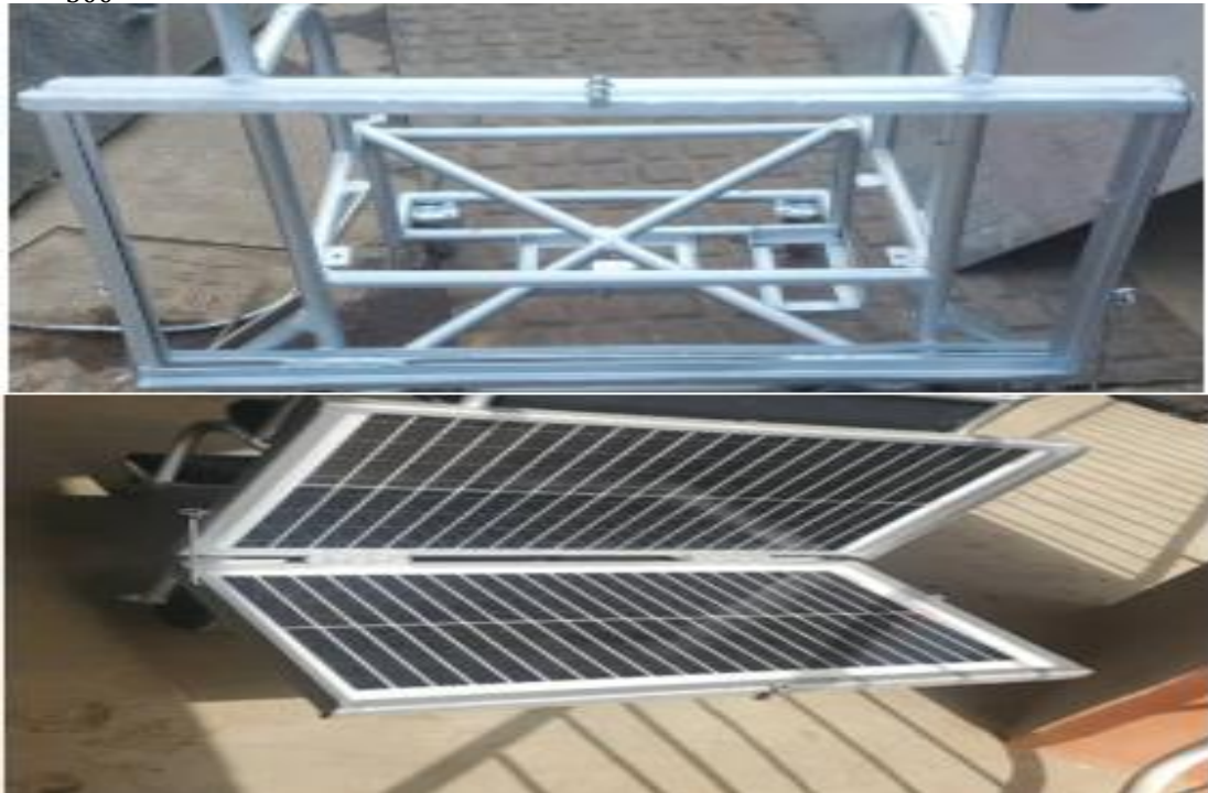
Figure 6: The solar panel carriers before and after solar panel installation
