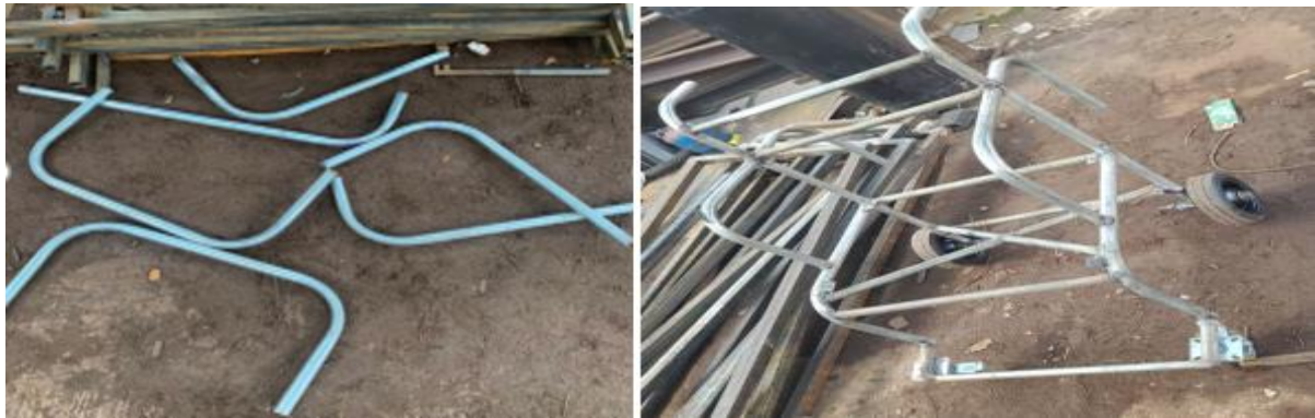
Figure 5f: Testing of steel iron AISI4130 for brittleness during bending
